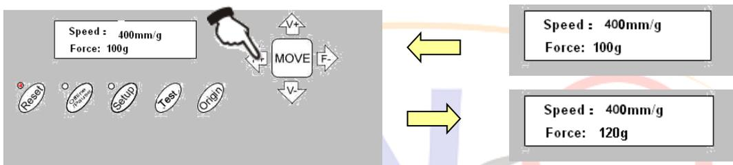
When it is working, if the RESET key is pressed, the machine will return to default settings and reset mode---clear up all information, and get ready for new work.
