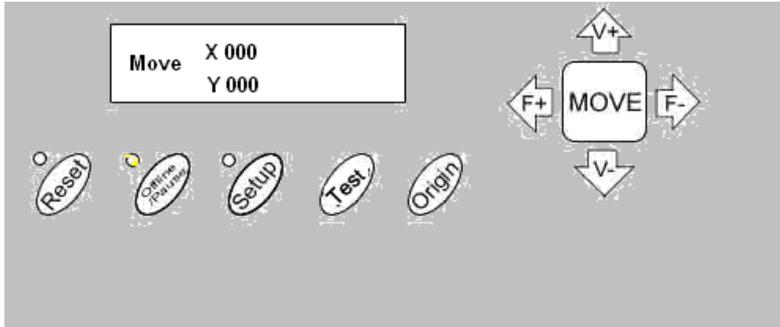
Press the key V+ or V- the carriage can be moved left or right. Press the key F+ or F- the vinyl can be moved forward or backward., In this state you can move the blade top to the starting position. the step value of “X, Y” in the LCD will change accordingly
