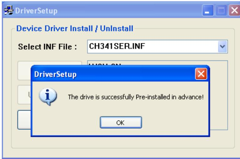
Now connect USB cable of the cutting plotter with USB port of computer . The USB device will be found as “COM3” from “ Device Manager”. It testifies that the machine is connected with computer successfully
